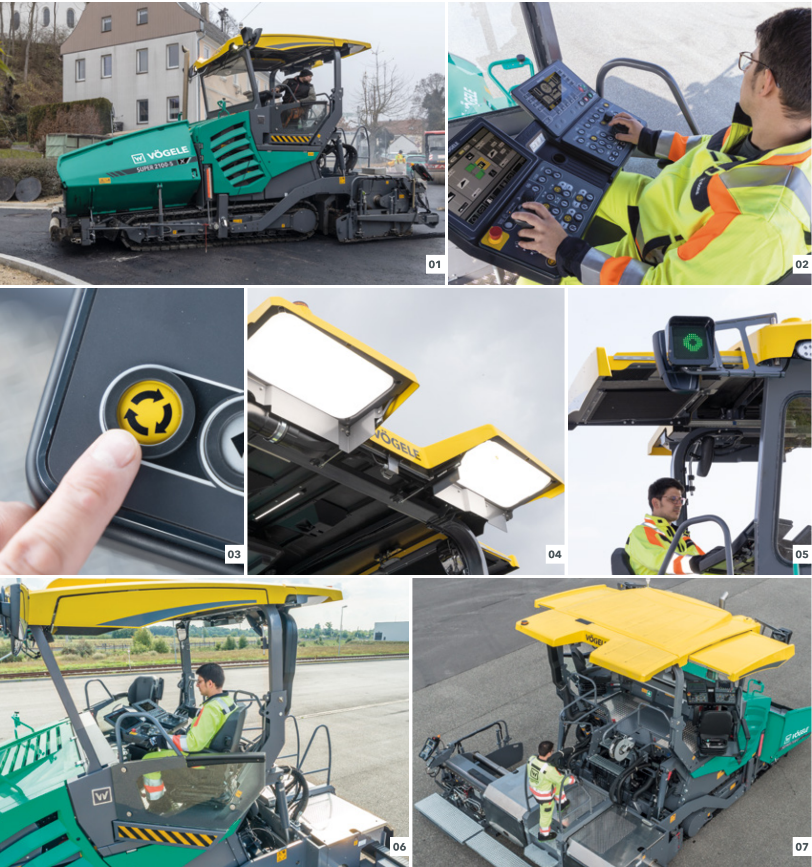
01 Pioneering, functional product design. 02 ErgoPlus 5 with many convenience and automatic functions. 03 Pave Assist Plus for easier repositioning on the job site. 04 Light Package Plus for optimum illumination of the screed operating area.
