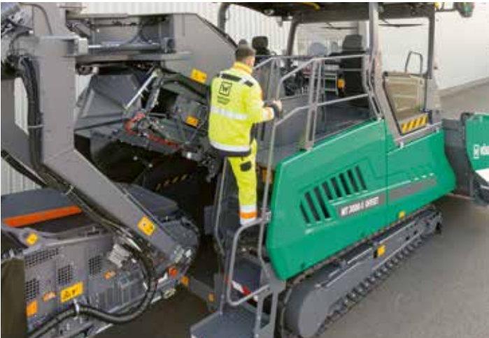
The comfortable ascent with handrail allows safe and convenient access to the spacious paver operator's platform.
